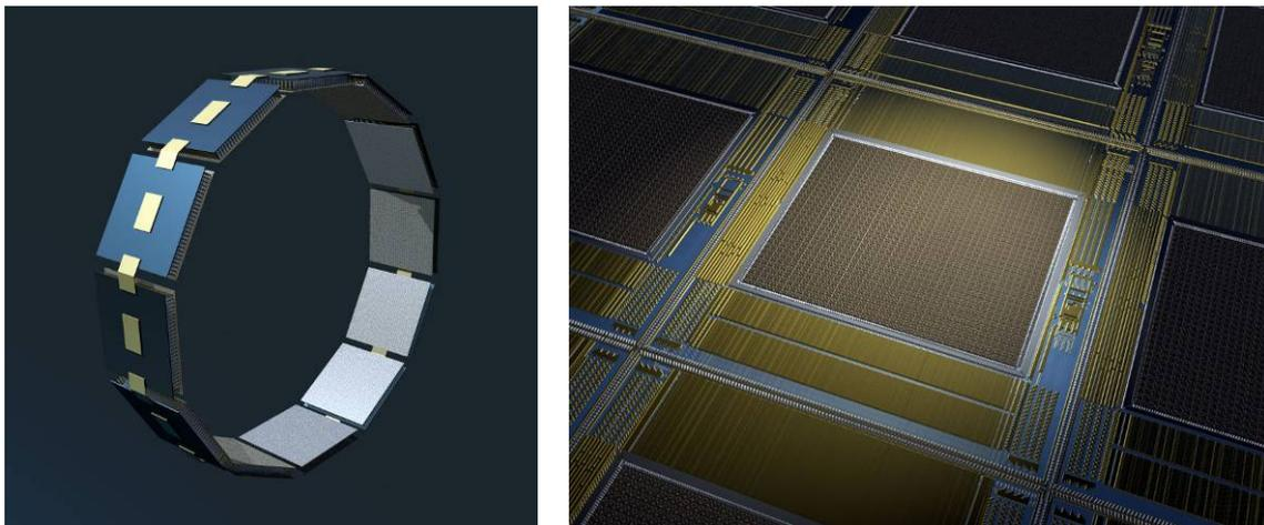
Figure 3. Left: Conceptual design of a possible SPADnet full pre-clinical PET implementation. Right: Conceptual layout of the SPADnet sensor array building up a single module (tessellating several tens of dies in abutment style using TSVs).
