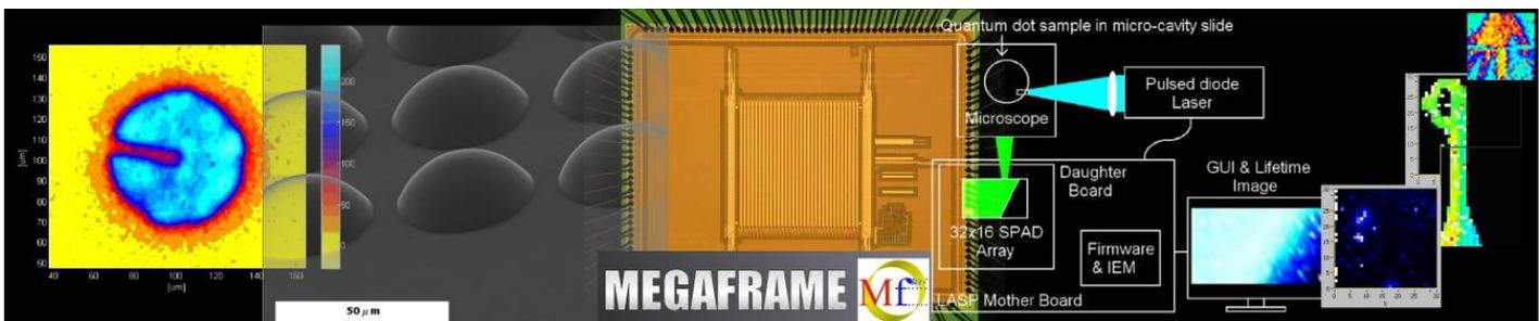
Figure 2. Main system features (bottom-up display). From left to right: SPAD pixel; microlenses; sensor array (32x32 version); system level overview; examples of results (lifetime images in selected applications)
