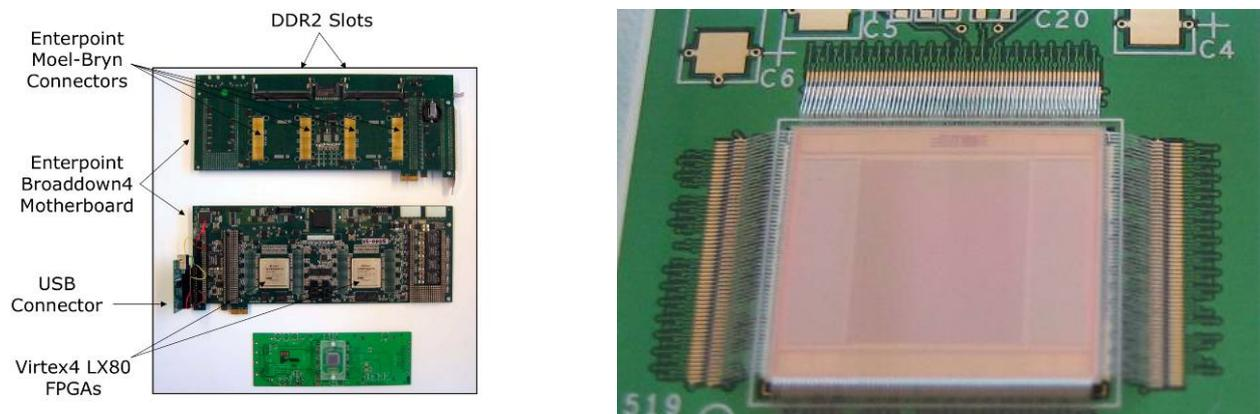
**Figure 1.** Left: FPGA card set for the 160x128 imager. The card set consists of an Enterpoint mother card with a dual VirtexIV FPGA and fast communication modules and a daughter card with a built-in chip-on-board. Right: Chip-on-board bonding of the 160x128 image sensor to the daughter card.
