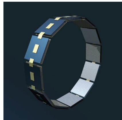
Left: Chip-on-board bonding of the MEGAFRAME 160x128 image sensor to the daughter card. Below: Main system features (bottom-up display). From left to right: SPAD pixel; microlenses; sensor array (32x32 version); system level overview; examples of results (lifetime images in selected applications). Right: Conceptual design of a possible SPADnet full pre-clinical PET implementation.
